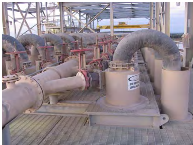
Figure 13. A hydrocyclone making a 150 mesh separation to remove clay minerals.
