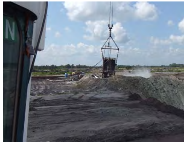
Figure 8. Water jets disaggregate the matrix and produce a slurry that is sucked into the large pipe (right center) and pumped by pipeline to a beneficiation plant.
